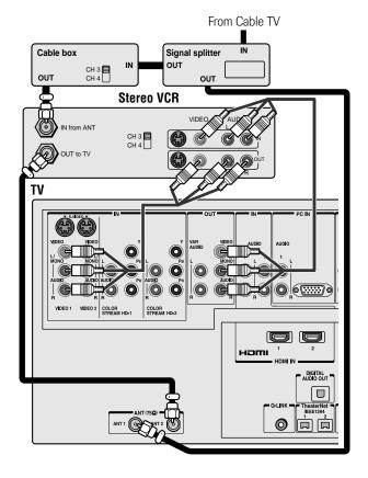
**Note:** The VIDEO/AUDIO OUT terminals output signals from the ANT 1, ANT 2, VIDEO 1, VIDEO 2, and VIDEO 3 terminals when the appropriate input mode is selected.
